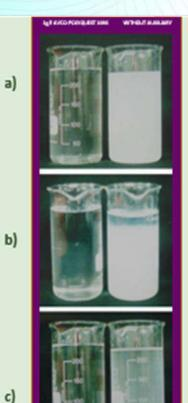
Demonstration of the efficiency of AVCO-POLYQUEST 1096 as a scale dispersing agent and as anti-precipitating agent (178 mg/I CaCO3)
