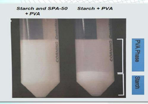
Blend of Starch and PVA are susceptible to separate in two phases. Addition of AVCO-SIZE SPA-50 eliminates this problem.
